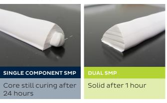
Bostik's Dual SMP system accelerates curing time and improves the green strength of adhesives and sealants in the initial hours following application.
